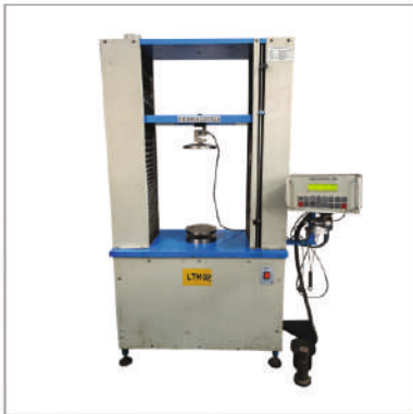
Load Testing Machine (Capacity : 500 kg)
